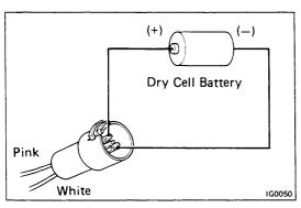
(c) Using a dry cell battery (1.5V), connect the positive
